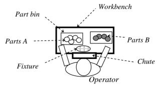
a) (2 points) The operator is sitting on chair and prompt to start his work as shown above. Then he move both hands simultaneously to part bins (left hand to left bin and right to right bin), grasp one part (both are light object) from each bins, move to fixture, place part A into fixture and place part B on top of A simulataneously (place parts to fixture by loose fit manner).
