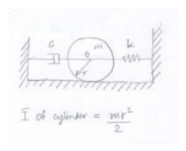
4. A designer wants to design a spring-damper shock absorbing system for his unicycle. The unicycle and its simplified model neglecting the mass of the unicycle are as shown. If the mass of the rider is 65 kg, and he designs to allow for 10% overshoot, and also wants the amplitude to reduce to 1% after 2 seconds, what are the values of the stiffness *k* and damping coefficient *c* he needs? (Hint: the ratio of two adjacent amplitudes are constant.)
