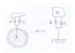
5. A refrigeration compressor is mounted on four springs of stiffness k = 200 N/m each, and has mass m = 55 kg, as shown. The mounts are made of spring steel with very low damping. Due to the design of the compressor, there is a vertical harmonic force of 12 N oscillating at the operating frequency of 1750 rpm. Determine the steady state vertical vibration of the compressor.
