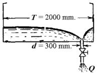
It is proposed to predict the minimum liquid level at which this entrainment can be avoided, at a draw-off rate of 150 m<sup>3</sup>/h, by model study in a smaller tank. For convenience, water at 30 °C (the density is 996.4 kg/m<sup>3</sup> and the viscosity is 0.8 mPa.s) is used for the fluid in this model study.
