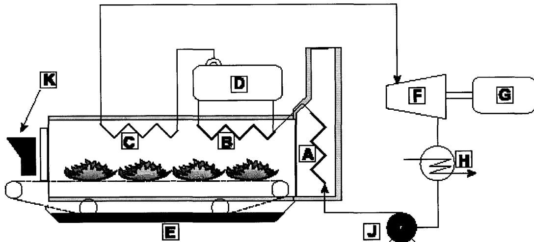
A moving-grate burner is used to generate superheated steam from wood waste. It is shown diagrammatically above. Give the names of the various items in the drawing
