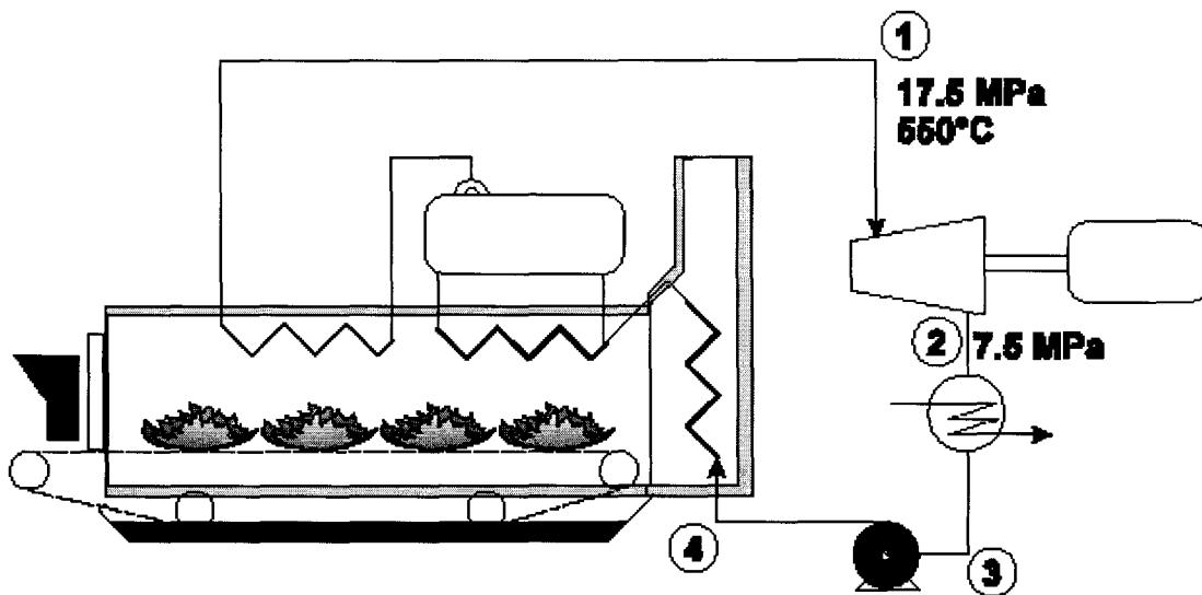
Steam at 17.5 MPa and 550°C is used to power a turbine/generator unit. It is exhausted at 7.5 kPa and condensed. The boiler feed-water is recompressed to 17.5 MPa before being re-introduced into the boiler.
