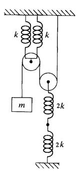
2. Determine the equation of motion of the system using energy method, and find the natural frequency of the system. The cylinder has mass m, and moment of inertia about its center of  $J_0$ .
