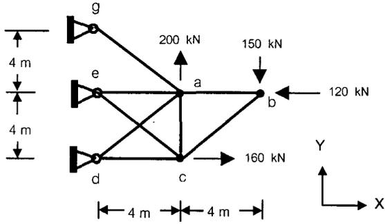
4. (30 คะแนน) Using the direct stiffness method (and neglect axial and shear deformation of members), establish the stiffness matrix, (matrix of order 4x4), for the plane frame shown below. And then determine all joint displacements of the structure. ( Given  $E = 2 \times 10^8 \text{ kN/m}^2$ , และ  $I = 6 \times 10^{-5} \text{ m}^4$  )
