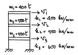
k, k, k are total lateral stiffnesses of the two columns of the storys as shown.
