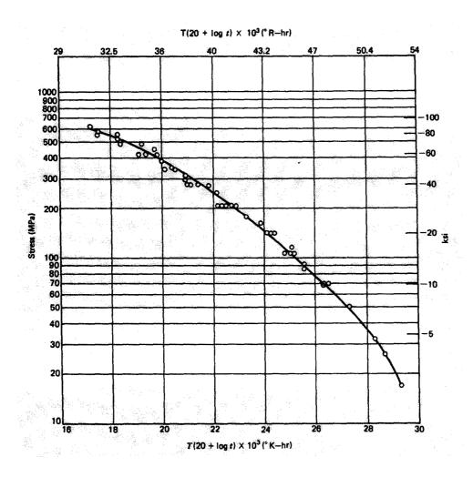
6.1 Determine the expected life for a sample tested at 500°C with stress 200 MPa. (10 points)
