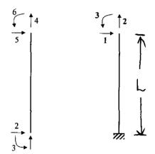
**Problem 3.** (15 points) Consider the structure shown below. (a) If you assembled the 10 x 10 stiffness matrix of the 10 unrestrained degrees of freedom and tried to invert it, what would happen? Why? (b) If you found the eigenvalues and eigenvectors (mode shapes) of the 10x10 stiffness matrix of the 10 unrestrained degrees of freedom, can you give one "easy" eigenvalue and sketch the corresponding mode shape?
