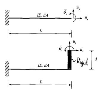
**Problem 2.** (30 points) Consider the two elements in the figure. The one to the left has rigid body modes; the one to the right is without rigid body modes. Find the transformation matrix  $\Gamma_{RBM}$  that governs the transformation between the two systems with the degrees of freedom numbered as in the figure.
