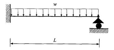
**Problem 5:** (30 points) The structure shown below was solved using the matrix displacement method ( $E = 200,000 \ MPa$ ). The resulting unknown displacements were found to be:
