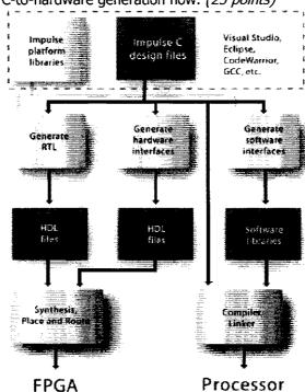
In this flow, design entry and initial desktop simulation and debugging are performed using common C development tools such as Visual Studio or gcc and gdb. The Impulse libraries provide the needed functions (as described in the preceding chapters) for software emulation of parallel processing.
