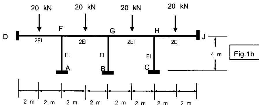
2. ( 25 ຄະແນນ) Determine the joint displacement components of the structures shown below, using the slope-deflection method.
