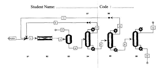
B3= separator B4, B5, B6 = distillation column B2 = reactor Stream Components methanol, toluene Feed hydrogen 5 8 methanol, recycle 11 toluene, recycle 12 styrene 13 ethylbenzene, water
