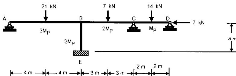
3. (30 ດະແນນ) Using the portal method, (an approximate lateral load analysis for frame structures), determine and sketch the bending moment diagram and the shear diagram for the structure shown below.
