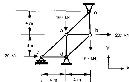
5. (25 ຄະແນນ) Using the direct stiffness method (neglect axial deformation of members), establish the stiffness matrix , ( matrix of order  $4 \times 4$  ), for the plane frame shown below. And then determine all joint displacements of the structure. ( Given  $E = 2 \times 10^8 \text{ kN/m}^2$ , และ  $I = 6 \times 10^{-5} \text{ m}^4$  )
