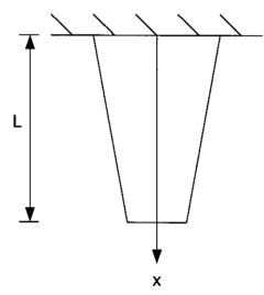
$\gamma$  = unit weight E = Modulus of Elasticity  $A(0) = A_0$   $A(L) = A_L$   $A(x) = A_0 - \frac{x}{L} (A_0 - A_L)$
