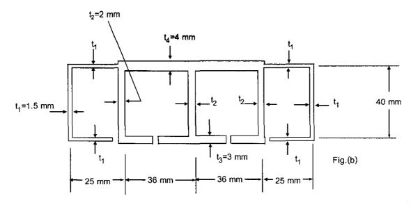
3. (25 marks) A steel member (E =200 GPa) with the cross section shown below is used as a cantilve beam of length L =2.0 m. The beam is subjected to a point load P = 12 kN at mid length passing through the shear centre of the cross-section, and with the direction as shown ( $\phi = 70^{\circ}$ ). Determine the maximum tensile and co appressive stresses in the beam and the deflection at the free end of the beam (C is the centroid of the cross-section).
