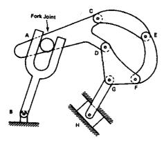
(b) Determine the mobility of this mechanism. How many kinematic inversions does this mechanism have, including the one shown in this figure? (6 points)
