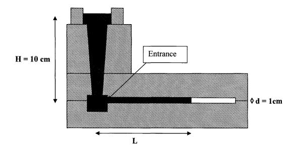
ii) If we pour the metal with the temperature 750°C, how far the metal will flow (L = ?) (10 points)?
