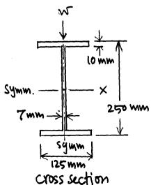
3. A hinged-hinged column is subjected to an axial load P as shown. Using the Rayleigh-Ritz method by assuming that the lateral displacement v in the y-direction for the buckling shape of the column is  $v = a \sin(\pi x/l)$ , determine the approximate elastic buckling load  $P_{cr}$  by the Rayleigh-Ritz method and compare the obtained critical load to the Euler buckling load. Comment on the comparison.
