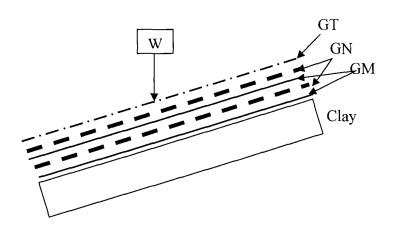
3. Calculate the tensile strain in a GCL as it deforms in an out-of-plane mode (as per the example problem of Section 6.3.3) for deformations of 0.10, 0.20, 0.30, 0.40 and 0.50 m. and plot the factor of safety. The allowable tensile strain of GCL is 14 %. The radius of the depression remains constant at 1.50 m. (10 points)
