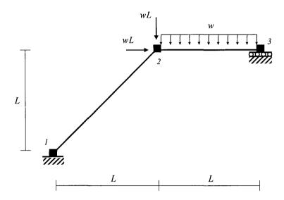
**Problem 4: (30 points)** Consider the truss shown below. Write down the matrix compatibility equations associated with free degrees of freedom.
