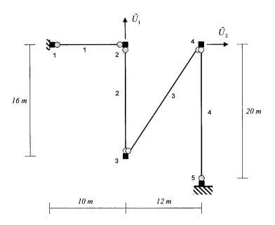
**Problem 6: (30 points)** Consider the beam shown. Using the strong form of the problem (beam differential equation + boundary conditions), find the end shears  $V_1$  and  $V_2$  and the end moment  $M_1$ .
