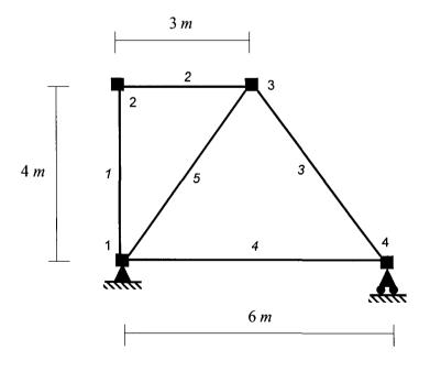
**Problem 5: (30 points)** With the assumption that all frame elements are inextensible, the mechanism in the figure below has two independent free displacement degree of freedom  $\tilde{U}_1$  and  $\tilde{U}_2$ . Determine the global displacements at all nodes corresponding to unit values of  $\tilde{U}_1$  and  $\tilde{U}_2$ .
