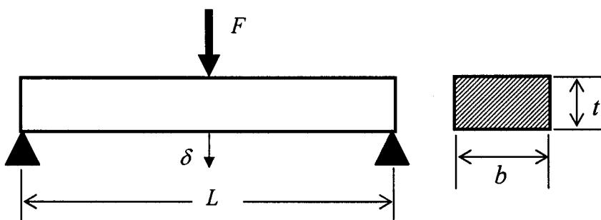
The mid-point deflection of an elastic beam of length  $L$  loaded in three-point bending by a central load  $F$  is given by
