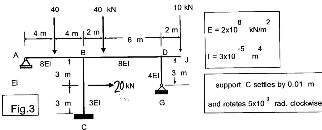
4. (30 ຄະແນນ) Determine all end moments of the frame shown below and draw its bending moment diagram (Hint: the successive sway correction moment distribution may be employed).
