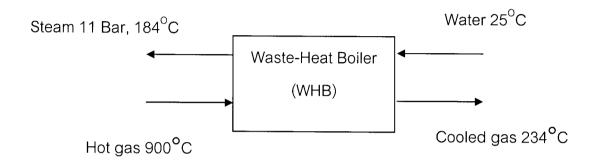
Hot gas component flow rates and temperature constant values for  $\boldsymbol{C}_{\!p}$  are:
