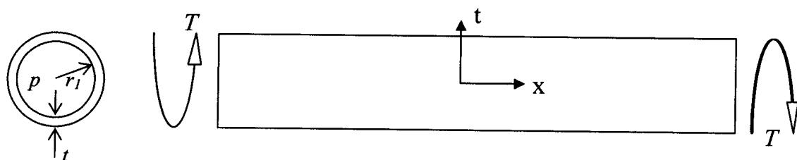
$$\text{Given: } \sigma_t = \frac{pr_1}{t}; \quad \sigma_x = \frac{pr_1}{2t}; \quad \tau_{tx} = \frac{T}{2\pi r_{avg}^2 t}$$
