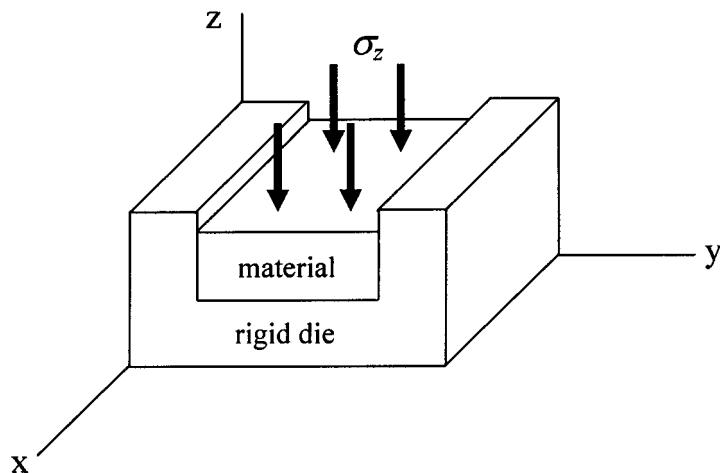
If  $\sigma_z$  has a magnitude of 75 MPa and the material is made of copper alloy  $E = 130 \text{ GPa}$ , and  $\nu = 0.343$ . Determine the followings:
