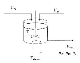
reaction rate constant k(T). For safety reason, the level of the tank should not less than 1/3 and higher than 2/3 of the tank height. And for economic reason, the concentration of  $x_C$  must be higher than 95%. If the operator accidentally, opened valve for stream  $F_A$  greater than its
