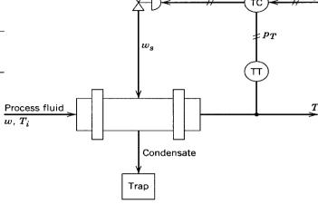
If PI controller (which Kc = 5.84 and  $\tau_I = 0.288$  min) is used in this process, calculate the corresponding gain and phase margins.
