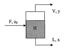
volatile component is fed to a single effect evaporator at a rate of F kg/hr. It may assume that vapor rate (V) and liquid rate (L) are constant and the liquid holdup in the evaporator is H kg. The dynamic mass balance can be written as,
