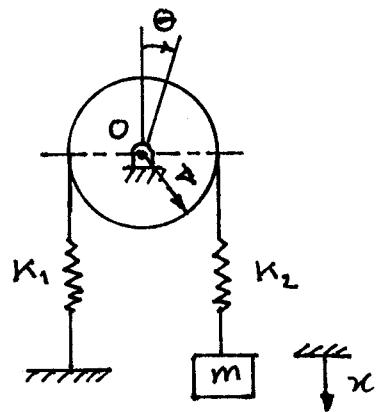
5. The equations of motion of a two degree of freedom system are shown below. Find the natural frequencies of this system.
