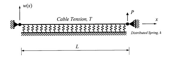
(a) Show that the governing differential equation of equilibrium (strong form) for the vertical displacement, w(x) of the cable in term of k, T, and P is:
