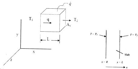
Consider the system shown above. The top, bottom, front and back of the cube are insulated, so that heat can be conducted through the cube only in the x direction. At x = 0,  $T = T_1$  and at x = L,  $T = T_2$ . Derive the temperature profile equation describing the temperature T as a function of x.
