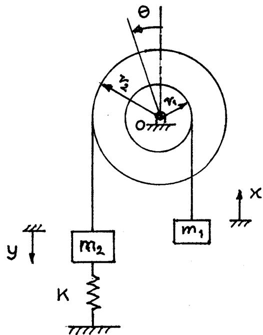
2. Determine the natural frequency of the pulley system shown below if  $W = 50 \text{ N}$ ,  $k = 900 \text{ N/m}$ . Assume the pulleys to be frictionless and of negligible mass.
