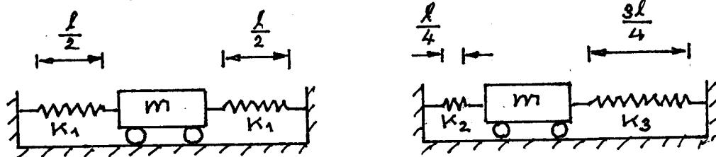
5. Determine the damping constant that make the system to be critically damped if  $m = 10 \text{ kg}$ ,  $k = 1000 \text{ N/m}$ ,  $x_0 = 0.1 \text{ m}$  and  $\dot{x}_0 = 10 \text{ m/s}$ .
