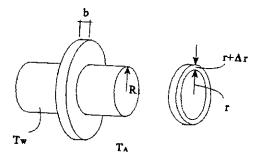
(a) Show that the steady-state heat balance on an elementary annular element of fin yields the equation
