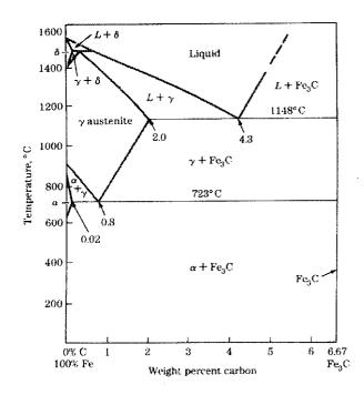
c) From the given phase diagram, draw the microstructure of a **0.5-wt% carbon** steel at room temperature. Also, answer how much of each phase in the microstructure? Show your work clearly (5 points).
