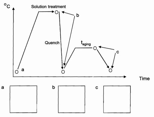
42. (4 points) From the diagram below, explain the effect of time and temperature of precipitation heat treatment
