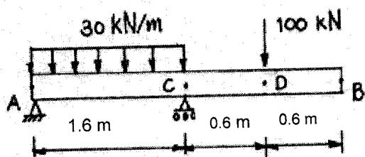
Question5 (10 คะแนน): For the beam and loading shown, determine the maximum tensile and compressive normal stresses due to bending.
