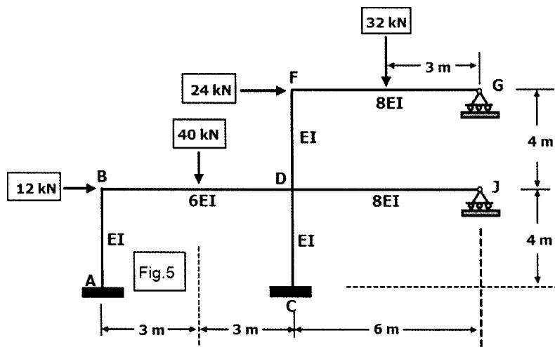
6. (25 points) determine end moments for all members of the frame shown below (consider the beam-column effects but neglect axial deformation effects). All relevant formulas for beam-column are given in the attached sheet.
