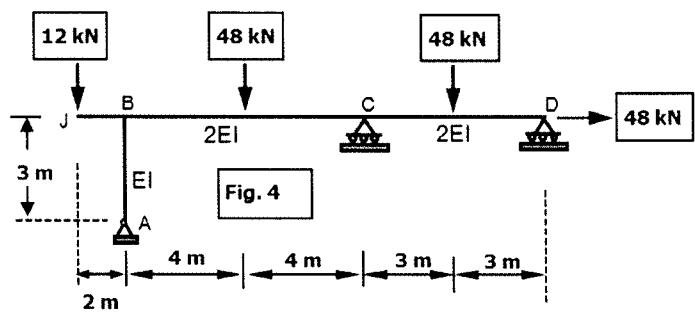
5. (25 points) Find all end moments of the frame shown below and draw its BMD (the successive sway correction moment distribution may be used, also note that flexural rigidity of the member BD is different from that of the members DJ and FG).
