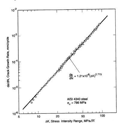
Given:  $N_f = \frac{a_f^{-(p/2)+1} - a_i^{-(p/2)+1}}{\left(-\frac{p}{2} + 1\right) A \sigma_r^p \pi^{p/2} \alpha^p} \qquad (p \neq 2)$  At fracture:  $K_{IC} = \alpha \sigma_{max} \sqrt{\pi a_f}$
