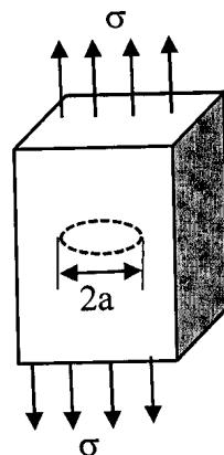
For an embedded penny crack:
