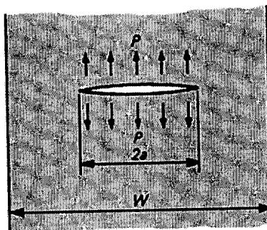
3.3 The fracture toughness for this steel is known:  $K_{IC} = 27.5 \text{ MPa}\cdot\text{m}^{1/2}$ . How high was the hydrogen pressure inside the crack at the moment of failure? (10 points)
