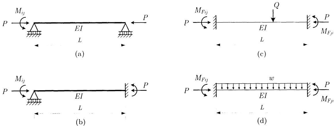
Rotational stiffness and carry-over factor with far-end pinned [Fig. (a)]
