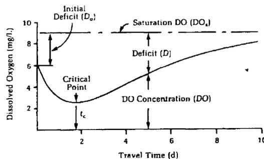
$$t_{crit} = \frac{1}{k_2 - k_1} \ln \left[ \frac{k_2}{k_1} \left( 1 - \frac{D_0(k_2 - k_1)}{L_0 k_1} \right) \right]$$
