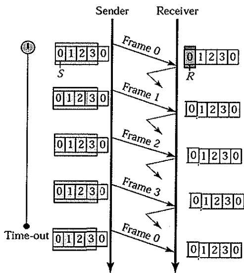
3. Below is Selective ARQ mechanism, it shows sending and receiving windows. Please put the pointer on the sending window (S) when the sender sends each frame out, and the receiving window (R) when the receiver sees each frame (10 marks)
